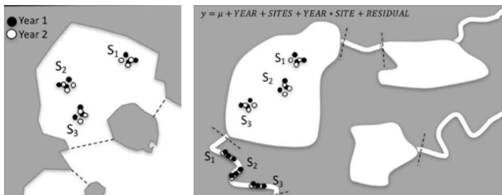
Figure 5.5: Schematics of orthogonal monitoring designs in a coastal water body (left) and in a lake and stream (right). In the examples, the number of sampled years, a = 2 , the number of sites per water body, b = 3 , and the number of samples per site and year, n = 3 . The generic mixed model of corresponding spatial and temporal factors is inserted in the right panel (modified from Lindegarth et al. 2013a).
